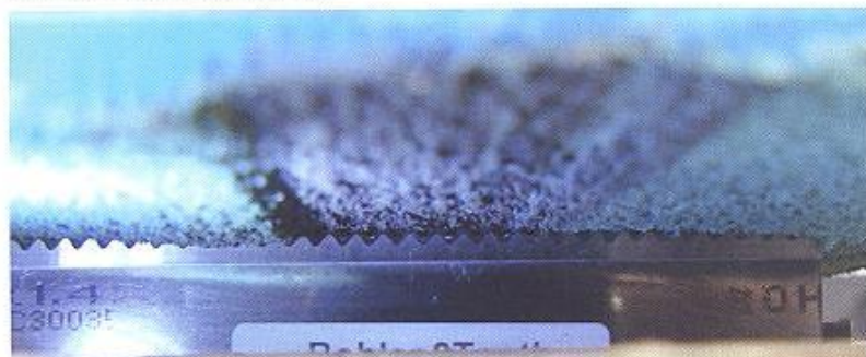
FIGURE 9, ABOVE: THESE "WHITE RUBBERS" ARE URETHANE SO WHILE THE ELASTIC RESPONSE FACTORS IN IT ALLOW FOR VERY QUICK REBOUND, OVER COMPRESSION AT RAPID CYCLES CONVERTS SOME OF THE ENERGY INTO HEAT, DESTROYING THE CELL'S STRUCTURE FROM THE INSIDE OUT.
