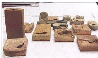
FIGURE 9, ABOVE: THESE "WHITE RUBBERS" ARE URETHANE SO WHILE THE ELASTIC RESPONSE FACTORS IN IT ALLOW FOR VERY QUICK REBOUND, OVER COMPRESSION AT RAPID CYCLES CONVERTS SOME OF THE ENERGY INTO HEAT, DESTROYING THE CELL'S STRUCTURE FROM THE INSIDE OUT.
