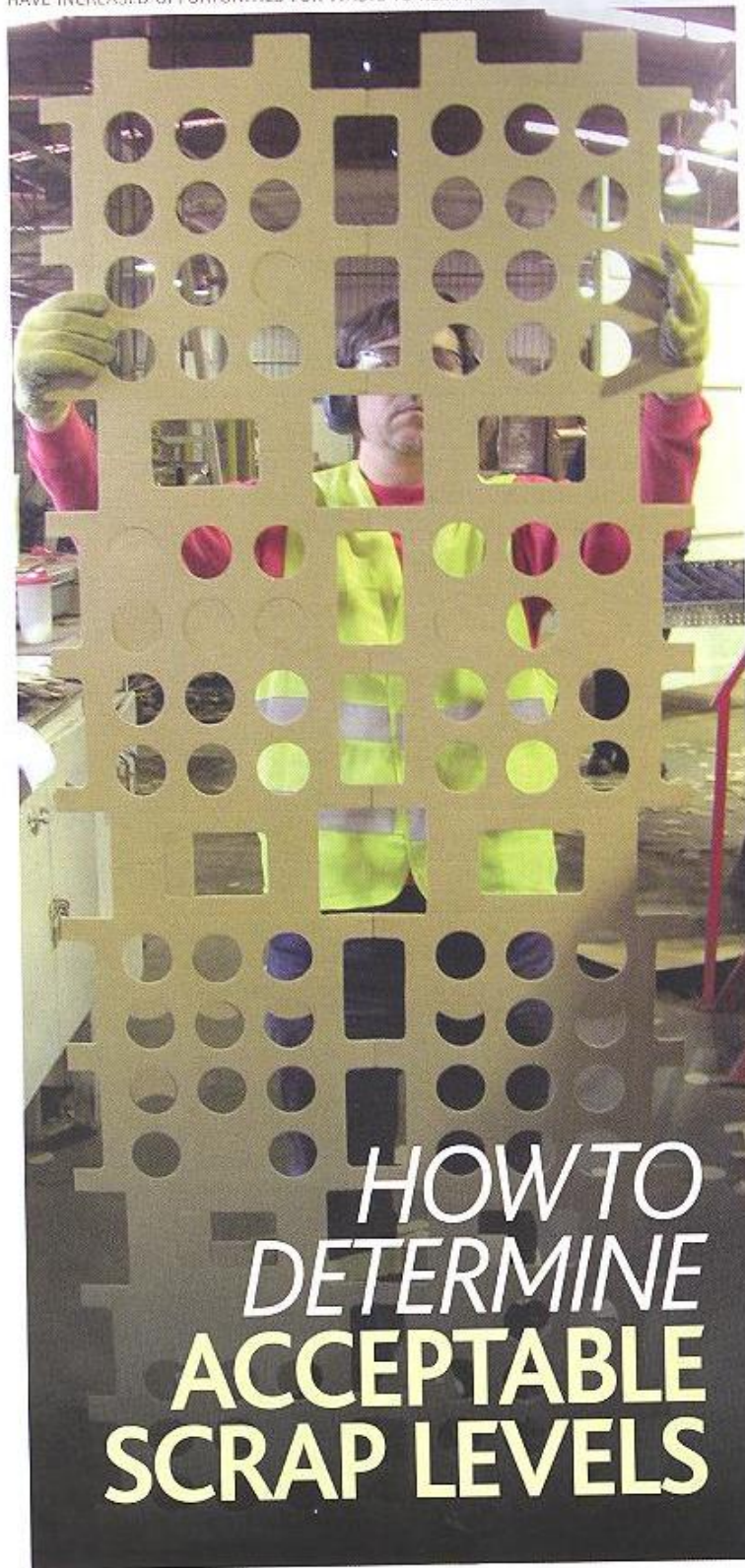
FIGURE 1: DESIGNS WITH A HIGH PERCENTAGE OF WASTE HAVE INCREASED OPPORTUNITIES FOR WASTE TO REMAIN.
