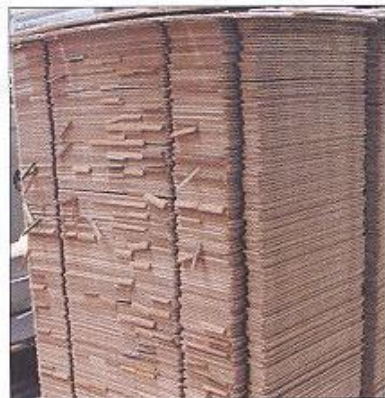
FIGURE 6: PLENTY OF TRIM WAS ALLOCATED, YET MOST OF IT REMAINED ATTACHED TO THE SHEET.
