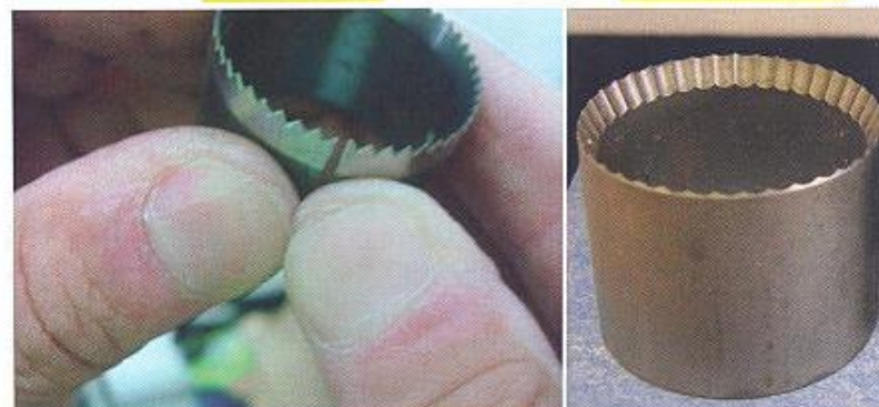
FIGURE 10, ABOVE: BENDING STEEL RULE INTO A CIRCLE WITH A SEAM THAT CAN SEPARATE IS NOT NEARLY AS EFFECTIVE AS A SEAMLESS PUNCH WITH AN INSIDE ABRUPT BEVEL.
