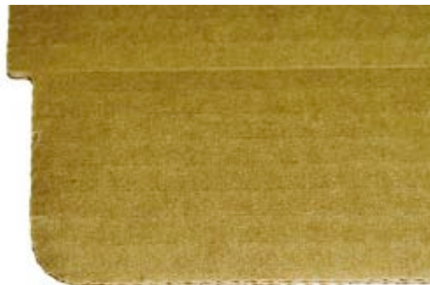
Below: Serrated "saw-toothed" edges are a telltale sign of rotary diecutting.
