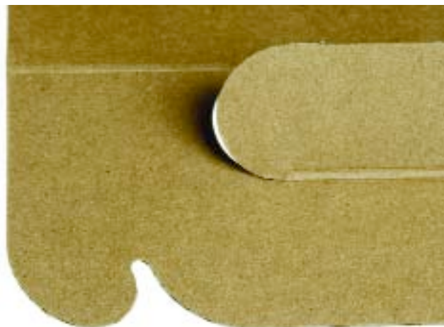
Above: Smooth edges produced by platen diecutting
