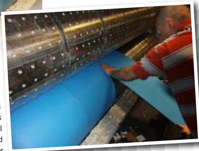
■ **Energy Return:** Also referred to as rebound. This is the ability of the cover to return to its previous state after being compressed. Proper rebound will result in the ability to use less impression to cut and clean the corrugated container, thereby allowing for minimal stress on the anvils, equipment and tooling.
