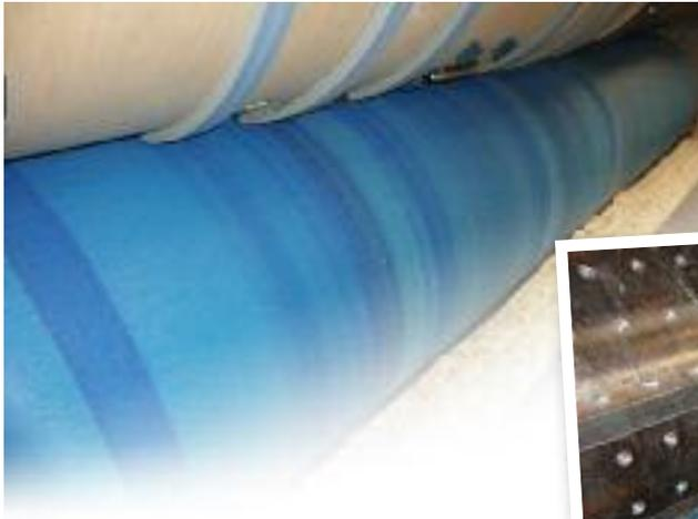
THE ANVIL COVERS WORK IN CONJUNCTION WITH THE DIE BOARD TO ENSURE PROPER CUTTING AND SCORING.
