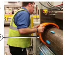
Slide one AnviLatch segment to the next cover position as shown.
