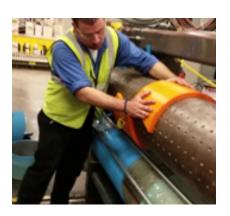
Install the female end of the cover (E) into the anvil cylinder slot directly in-line with the AnviLatch sleeve.
