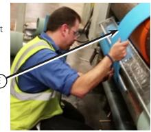
Rotate the cylinder approx. 180 degrees and slide the second AnviLatch segment to the next cover position as shown.
