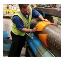
If necessary, adjust the nip height so the Anvilatch sleeve makes contact with the anvil cover surface.
